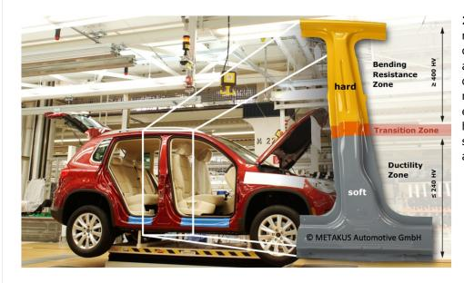
**2006**: First application of a thermomechanically tailored body component in large-scale automotive production; the highly ductile foot section of the B-pillar reinforcement enables controlled energy absorption, while the ultrahigh-strength center and head sections provide intrusion resistance and rollover stability
